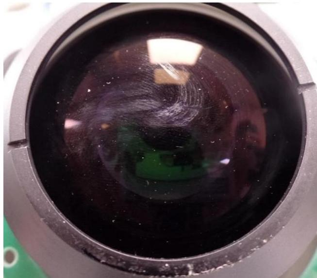
**Figure 2.4 Maestro – Dusty and smudged objective lens**
