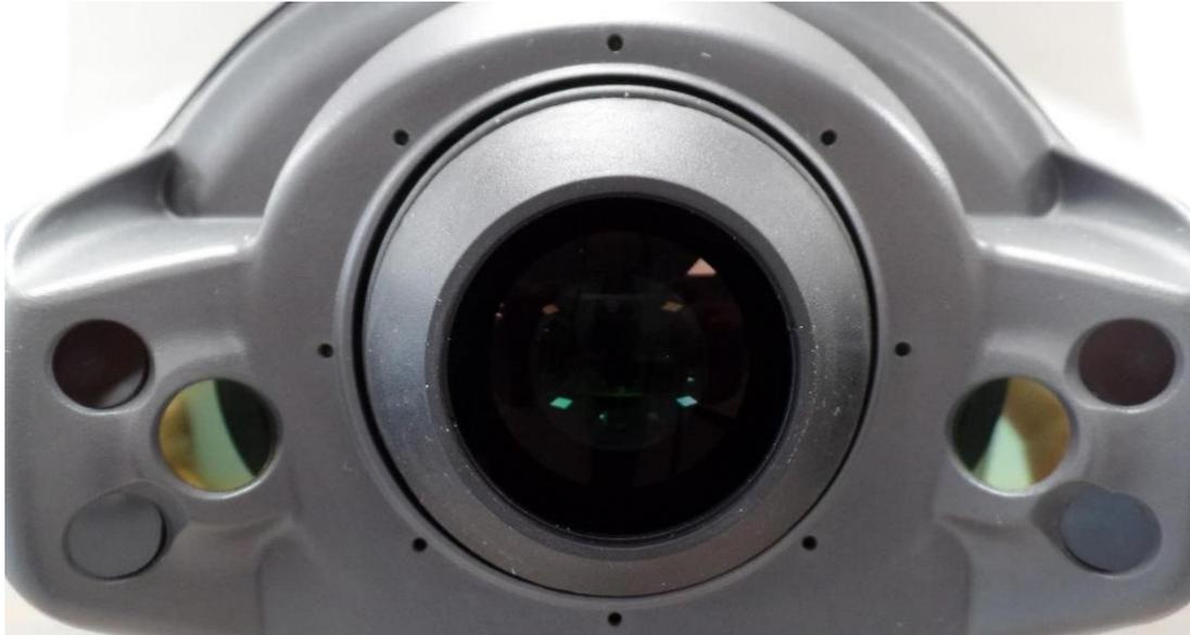
**Figure 2.5 Maestro – Cleaned objective lens and filters**
