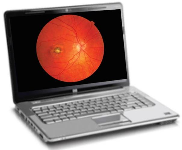
The wireless review station can be left permanently in an exam room or can be mobile from room to room in a 30ft. radius. Commercially available monitor, keyboard and mouse can be added by the user for his/her convenience.
